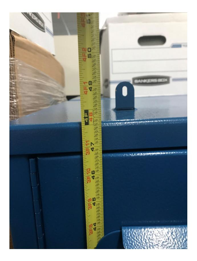
Current kiosk specifications: Exterior: Height w/o sign: 47.81 in. Height w/ sign: 68 in. Width: 18 in. Left Side with Door Extended: 36 in.
